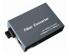
Protocol: IEEE802.3U IEEE802.3 Interface: RJ45 (10/100Base-TX) SC / ST / FC (100Base-FX) Mode: MM, SM Wavelength: 1310nm/1550nm Transmission Distance: 1310nm, 2~80KM; 1550nm, ~120KM Transmission Power: -14dBm~ -3dBm Receiving Sensibility: -31dBm~ -35dBm Saturation of Light: -14dBm~ -3dBm
